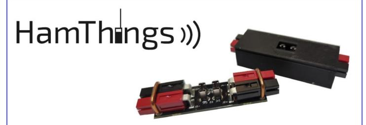
Chris N9CVR has is selling Powerpole Fuse Blocks. They are designed for mini APM/ATM blade fuses, up to 30 amps. Each Fuse Block weighs only 0.8oz!
